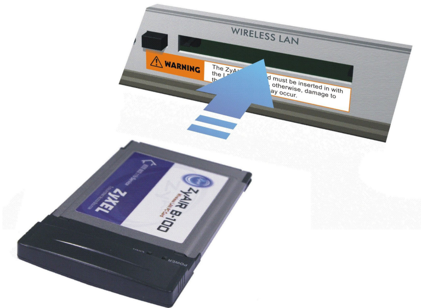
Figure 2-9 Inserting the Wireless LAN Card
