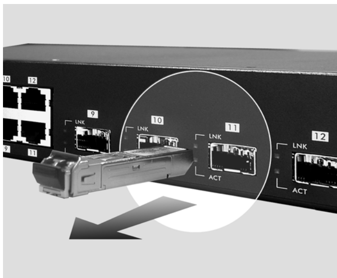
Figure 3-5 Transceiver Removal Example
