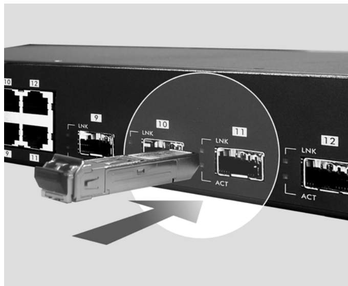
Figure 3-2 Transceiver Installation Example
