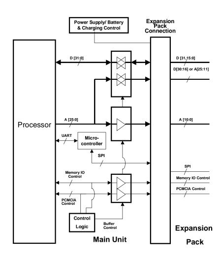
FIGURE 2: Expansion Pack Interface on Main Unit
