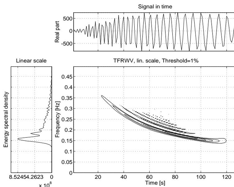
Figure 4.30: WVD of a bat sonar signal
