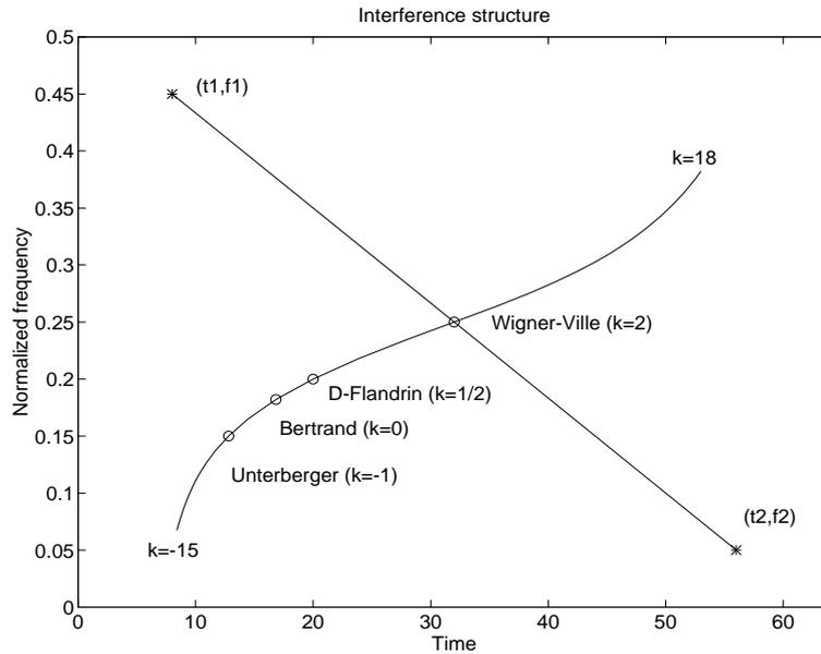
Figure 4.26: Locus of the interferences between 2 points for the affine Wigner distributions (parameterized by  $k$ ). For  $k = 2$ , which corresponds to the Wigner-Ville distribution, we obtain the geometric mid-point
