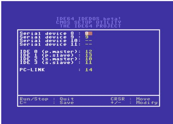
Figure 4: Device number setup
