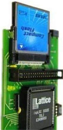
Figure 1: IDE64 V3.4 with CompactFlash
