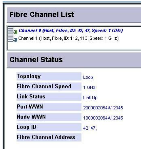
Figure 11-10: Fibre Channel Status Window
