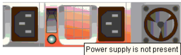
Figure 13-10: Faulty PSU Module Message
